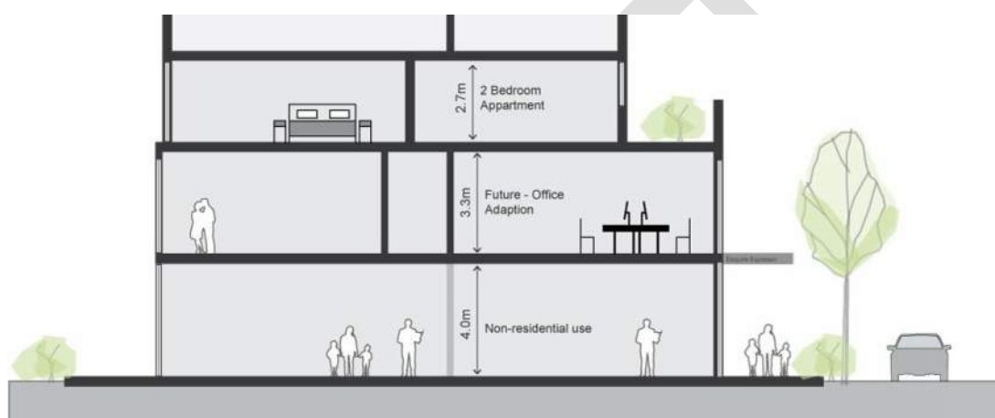
Figure 49: Building cross section showing higher ground floor and potential commercial use
