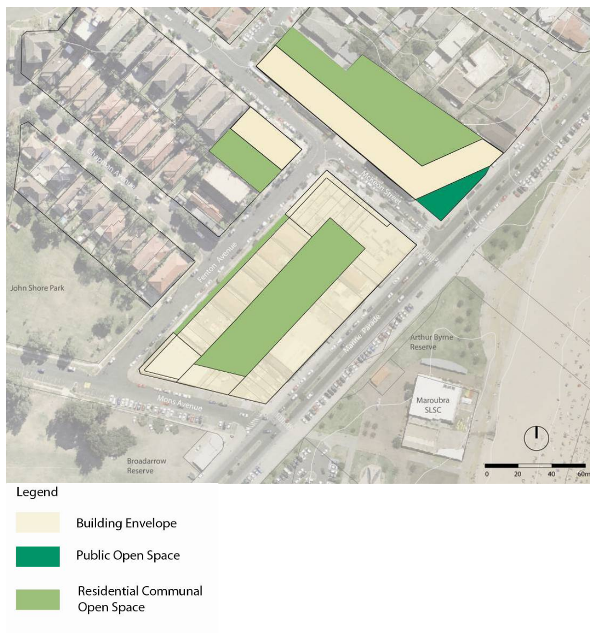
Figure 15 Open Space Base Scheme
