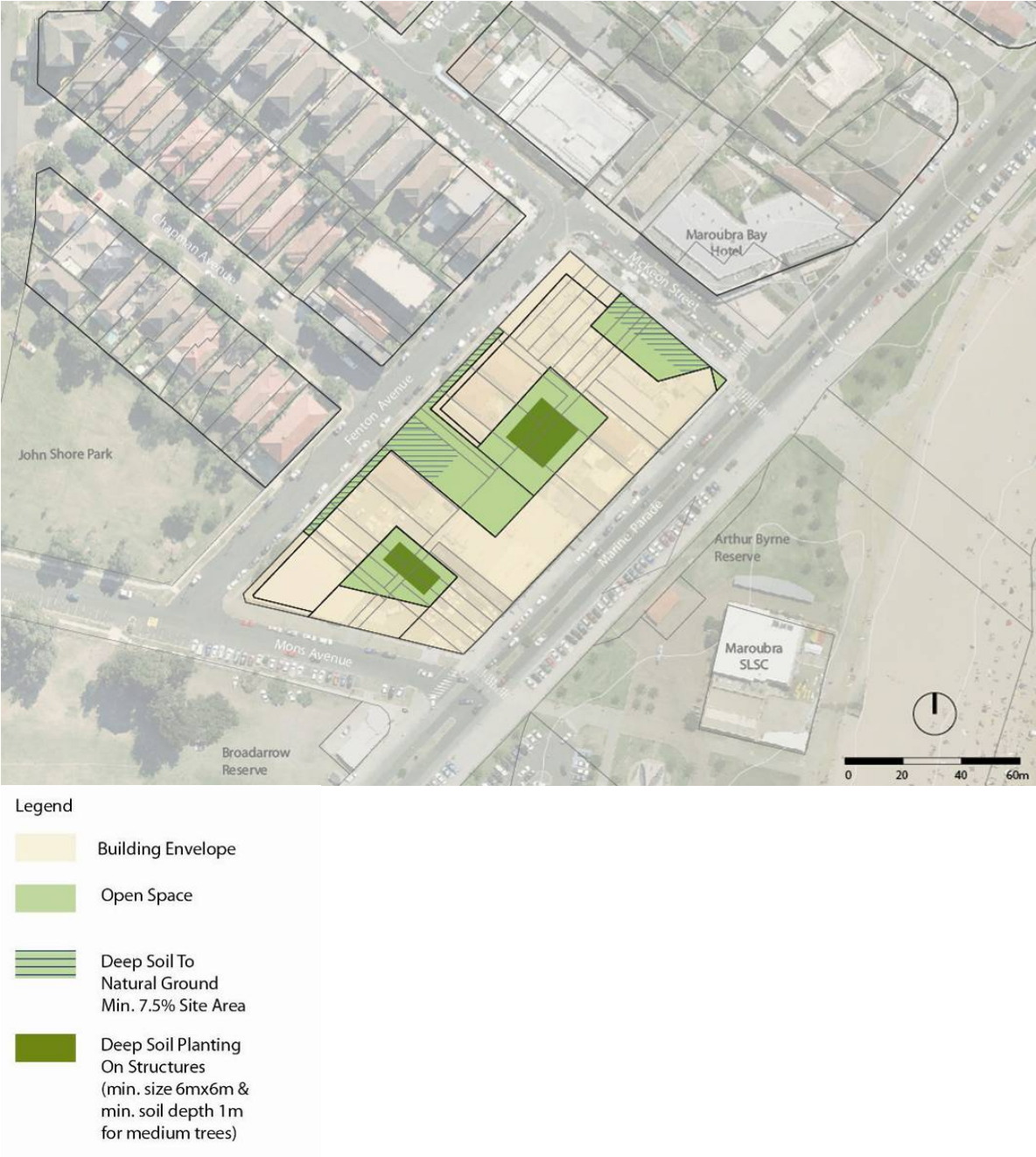
Figure 16 Deep Soil Zone landscape Requirements – Amalgamated Scheme
