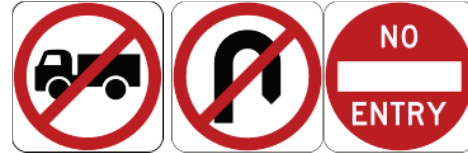
Figure 38: Examples of Prohibited Movement Signs
