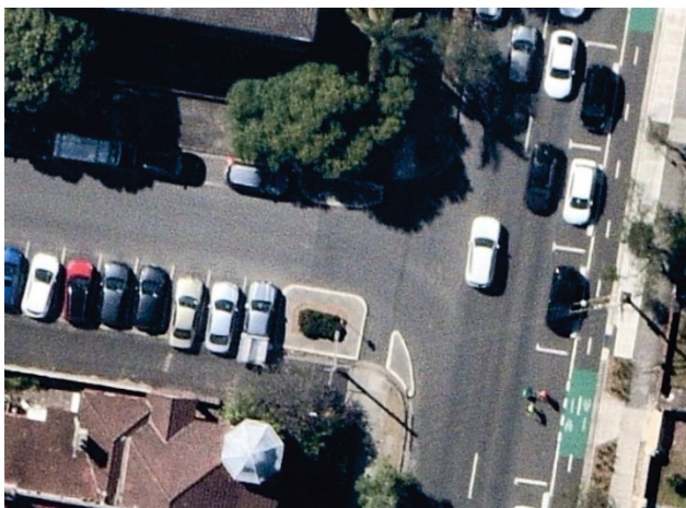
Figure 26: Lane Narrowing/ Kerb Extension
